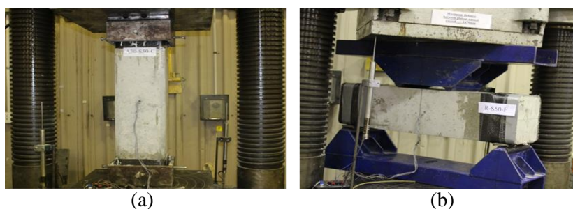
Figure 1. Test setup: (a) Axial compression and (b) Four-point bending
