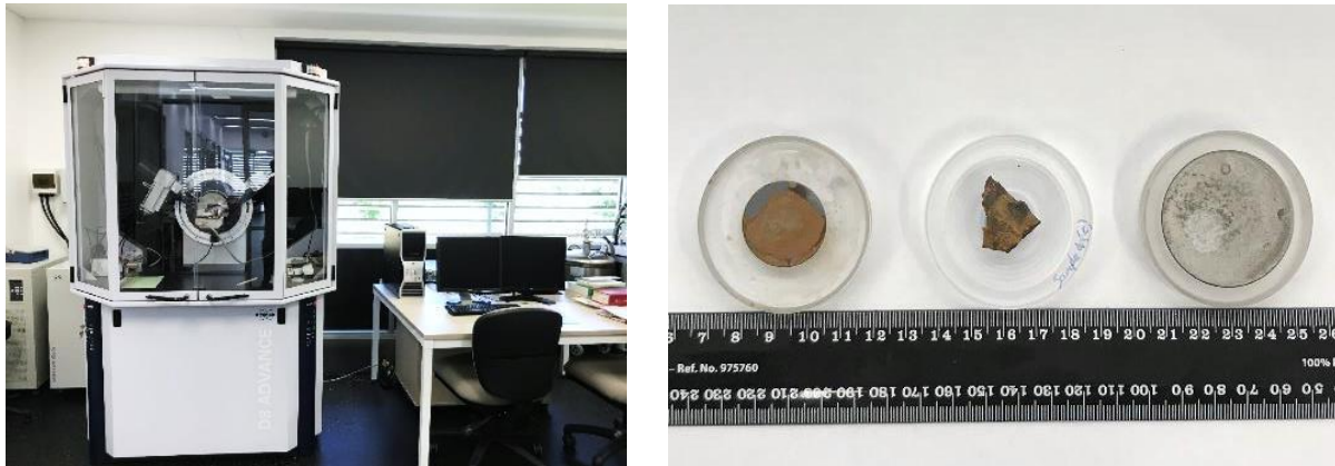
Figure 5. a) X-ray diffraction (XRD) instrument and b) sample preparation for the XRD
