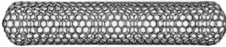
Figure 2: Closed single-walled carbon nano-tube [8].
