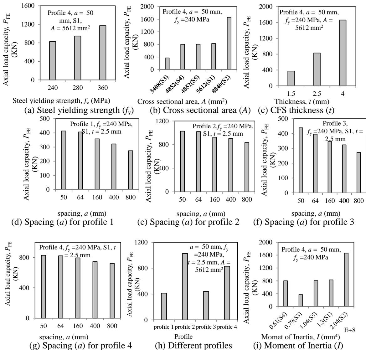
Figure 4. Effect of different parameters on CFS built-up stub columns.
