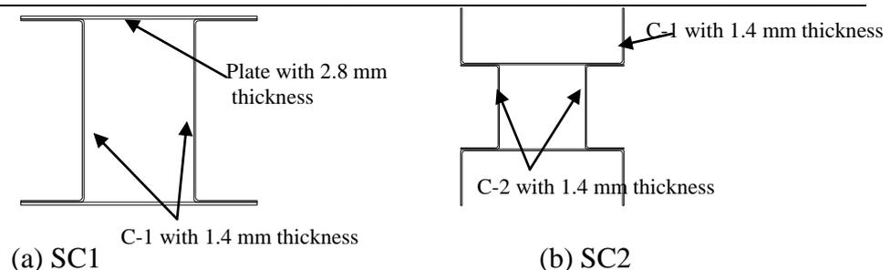
**Figure 2. Columns profile used by Meza et al. (2015)**
