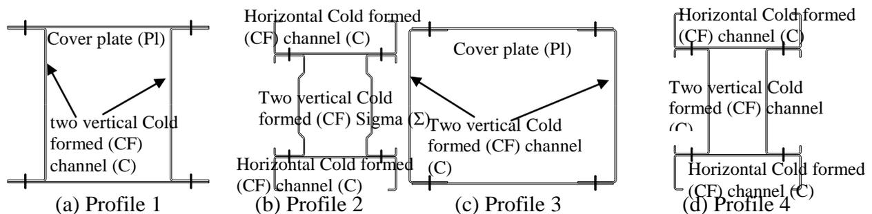
**Figure 3. Four Different profiles used in the parametric study.**
