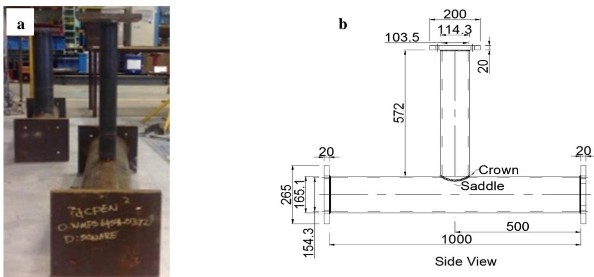
Figure 1. (a) T-joint specimens; (b) Figure 2. (a) T-joint specimens; (b) dimensions of T3 dimensions of T3 specimen
