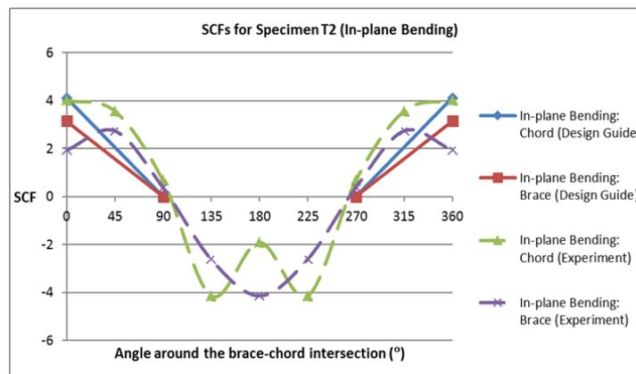
Figure 7. SCF distribution of specimen T2 under in-plane bending along chord/brace intersection
