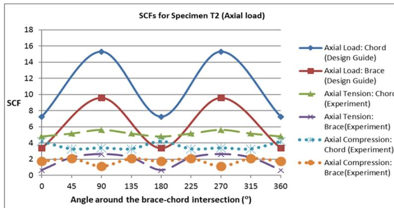
Figure 5. SCF distribution of specimen T2 under axial load along chord/brace intersection
