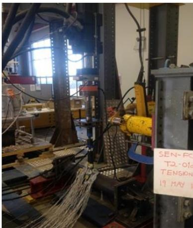
Figure 3. Test set-up for axial loading
