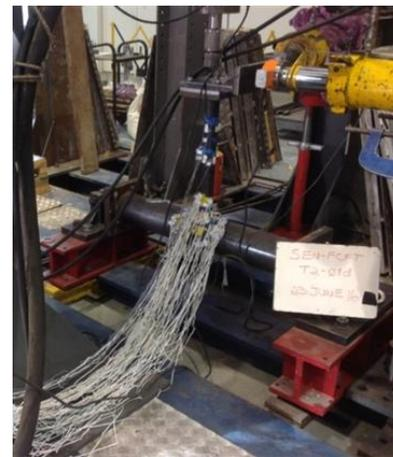
Figure 4. Test set-up for in-plane bending
