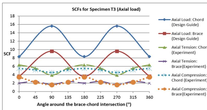
Figure 6. SCF distribution of specimen T3 under axial load along chord/brace intersection
