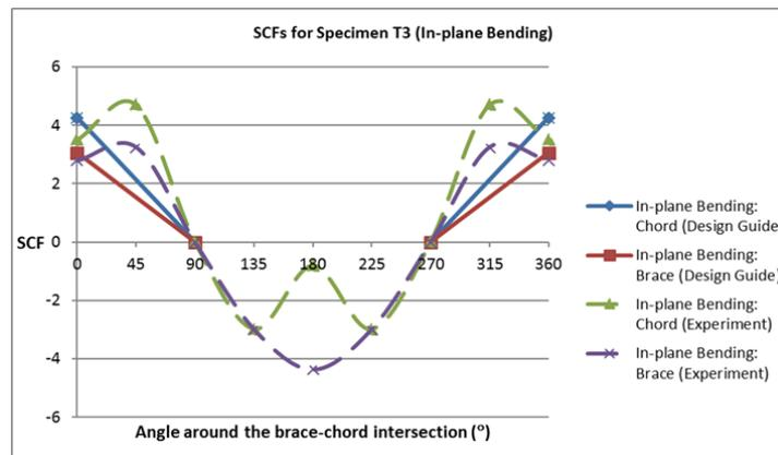
Figure 8. SCF distribution of specimen T3 under in-plane bending along chord/brace intersection
