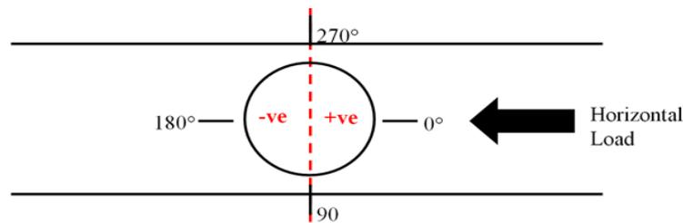
**Figure 9. T-joint under in-plane bending**
