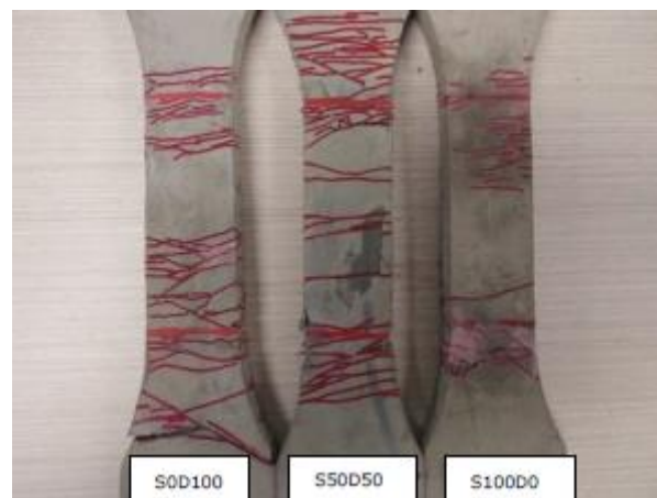
Figure 3. Crack patterns of the specimens
