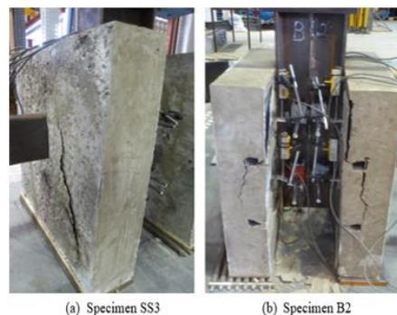
**Figure 6. Governing failure mode examples.**
