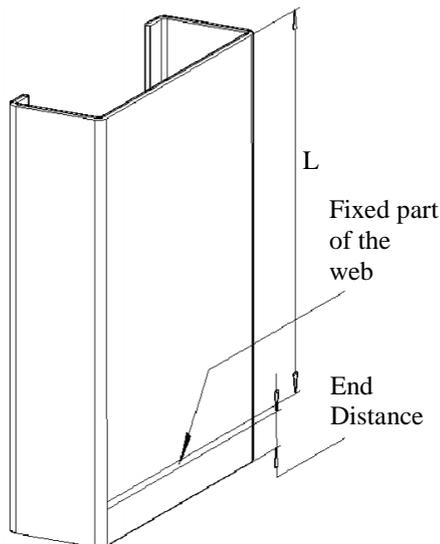
Figure 1 End distance and length of column
