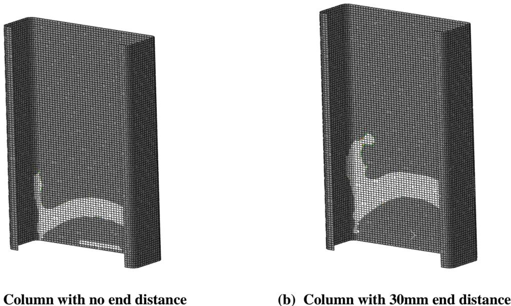
Figure 4 Stress distribution of yielded area in bottom port of the column
